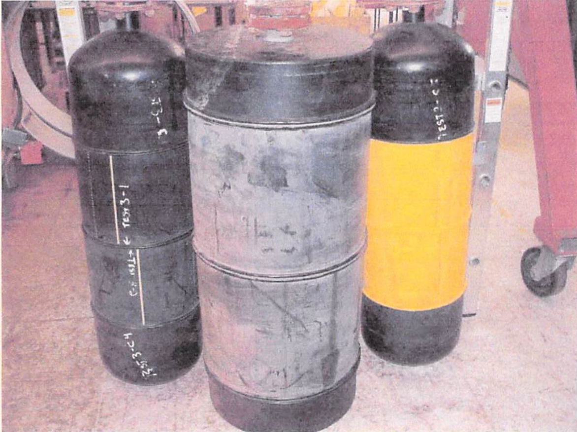
Photo 1 shows, left to right, one tested specimen from Test III (PE100), Test I (PE3408), and Test II (PE2406) samples.
